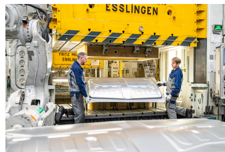
Sono Motors Ongoing Construction of 37 Sion Series-Validation Vehicles and Bodies in White
