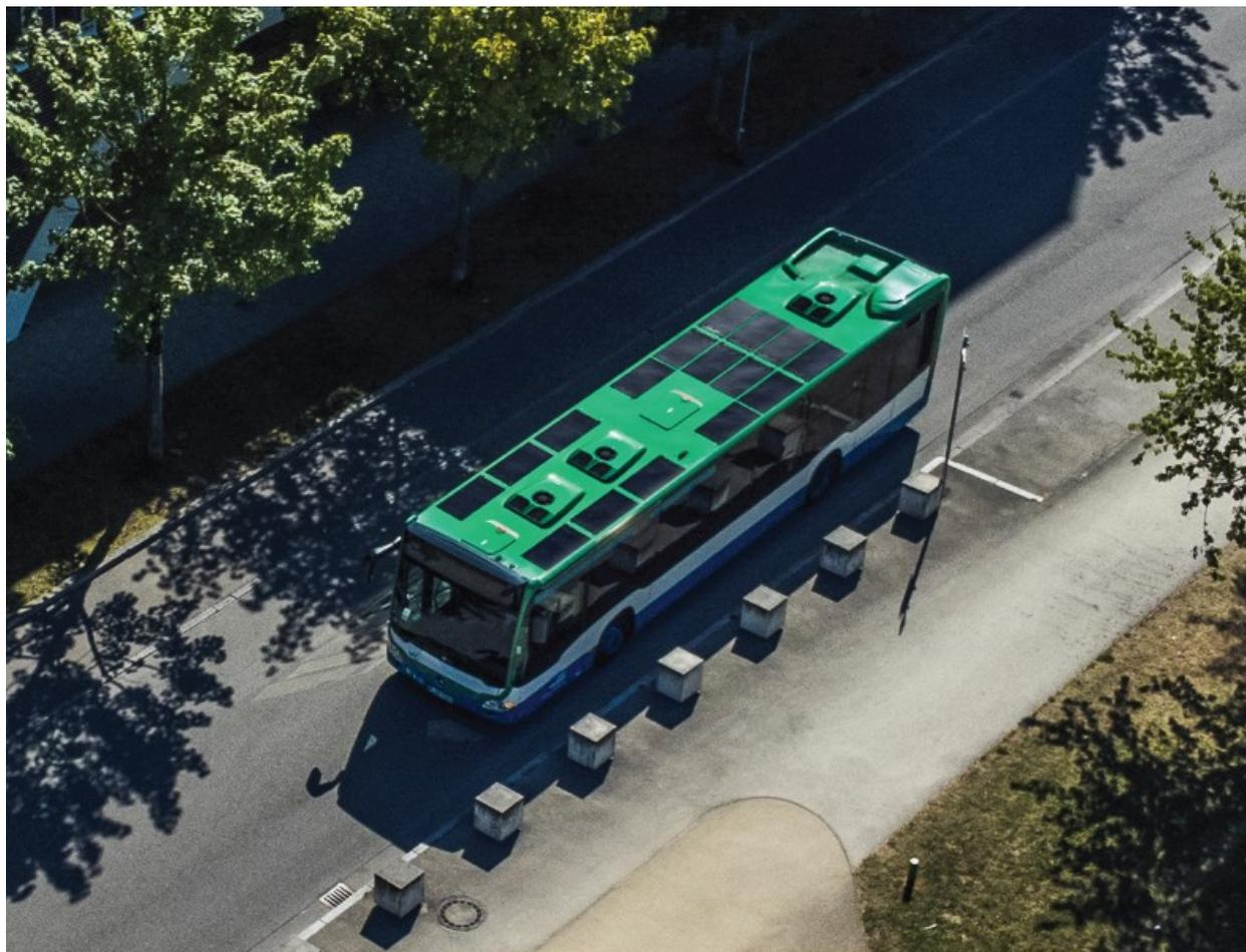
The Solar Bus Kit allows subsystems like the heating, ventilation and air conditioning to be partially powered by renewable energy thereby saving fuel, CO2, and costs. The Solar Bus Kit can save up to 1,500 liters of diesel and up to 4 tonnes of CO2 per bus
